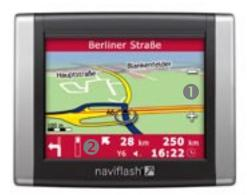
If you operate the navigation system via the touchscreen function, it will become dirty over time and both the readability of the information on the display and its input functionality will deteriorate.
